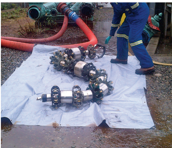
PICA’s SeeSnake tool can find weaknesses through liners and cement, whether the pipe is ductile, cast, or steel. The tool works by sending a signal throughout the pipe and reporting a time lapse that indicates thinning and thickening pipe walls. (Photo Courtesy of Bill Jappy)
